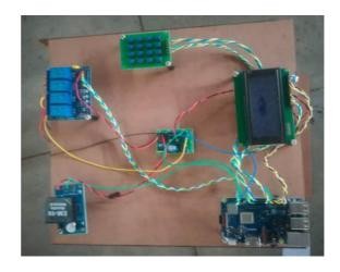
The system has raspberry Pi microcontroller which is 8 bit RISC microcontroller board which control the functionality of all the component in this system. The system is connected with hardware components like RFID module, keypad module, LCD module, NodeMCU module, and dispenser box.
